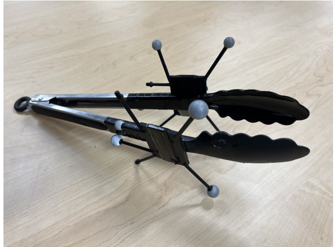
Fig. 2: Instrumented tongs utilized in the ARPOC-LfD system. The tongs are tracked using the OptiTrack motion capture system via infrared markers. The two distinct groups of markers enable the system to detect a closed gripper based on the center-point distance between the groups.
