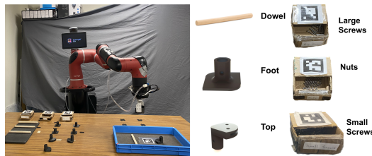
Fig. 2: Left: the experimental task setup. The Sawyer robot attempts to move construction components from the left of the table into the blue bin on the right, pushing the bin forward to deliver it to the human. Right: the components Sawyer can deliver as part of its sub-tasks.
