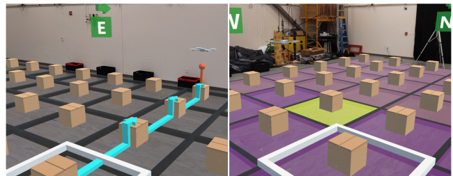
Figure 1: AR-based interfaces for prescriptive (Left) and descriptive guidance (Right) in the Minesweeper domain. In the prescriptive condition, suggested moves are shown as cyan arrows between grid squares, with suggested defuse actions indicated by the orange pin (underneath the virtual drone teammate). In the descriptive condition, grid squares are colored as a heatmap, representing the probability for each square containing a hidden mine as judged by the drone, from dark purple (low) to bright yellow (high).
